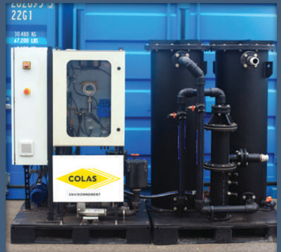
Figure 2 - Skid de Venting
